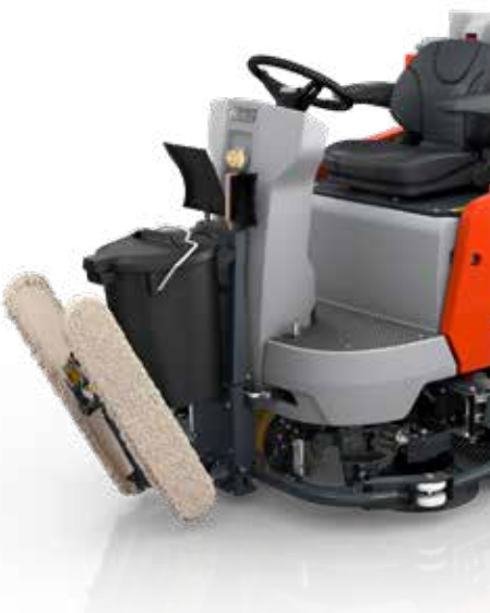
When not in use, the tools "mop" and "broom" can swiftly be folded up and out of the way.
